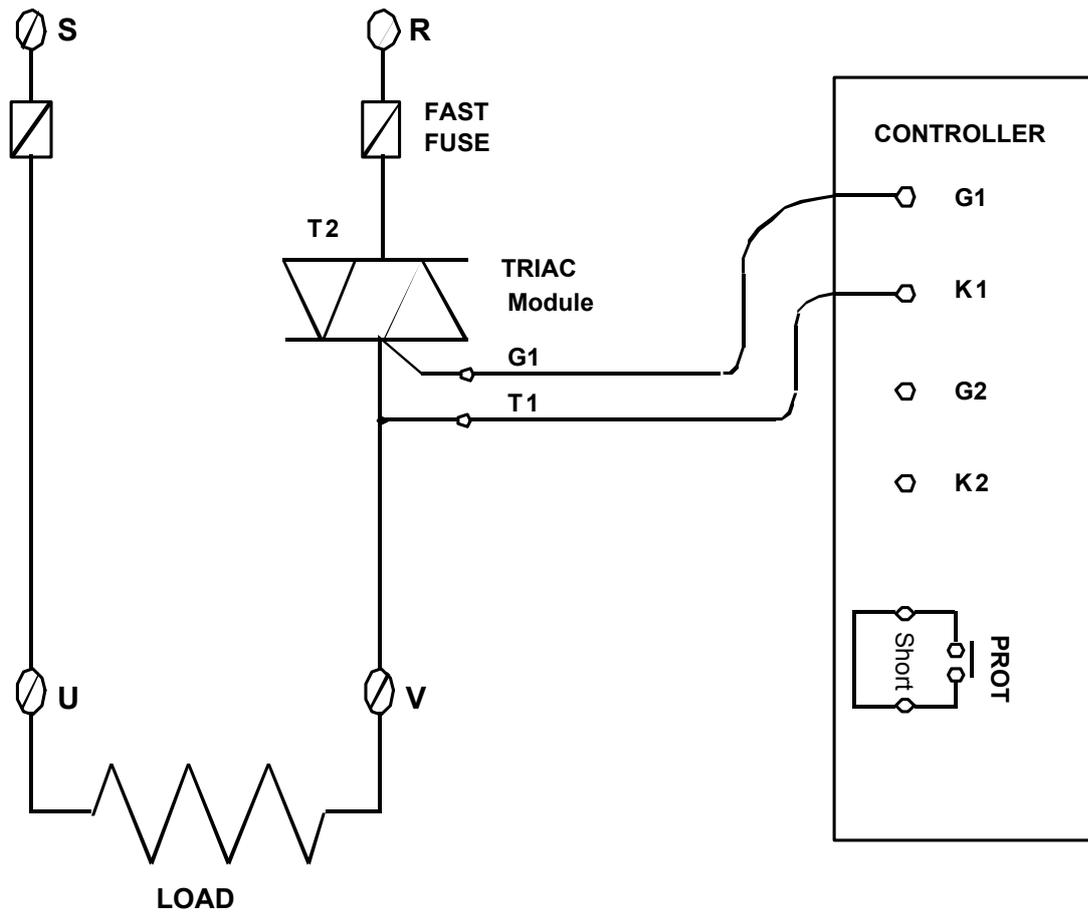
\*\* Controller source phase must be same as load source phase
