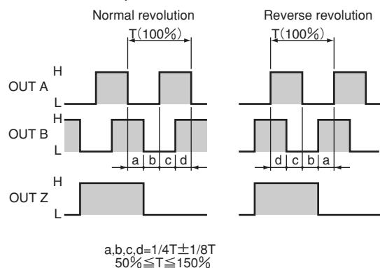
The above waveforms apply to normal (clockwise) revolution viewed from the shaft.
