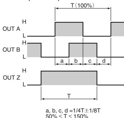
The above waveforms apply to normal (clockwise) revolution viewed from the shaft. OUT Z phase is reversed on the RZL and RZWL models.
